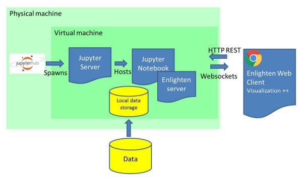
Figure 1. System architecture for VRE established in the EPOS Norway project.
